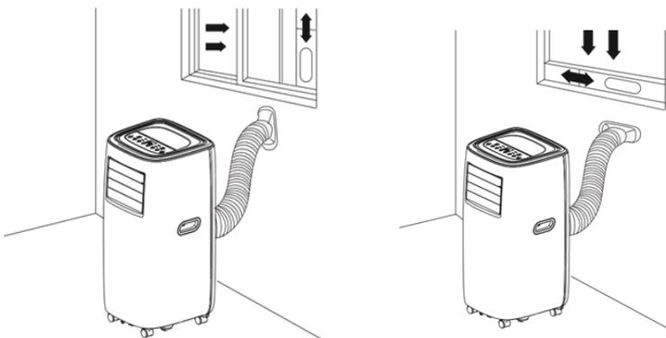
1. Partially open the window and place the extended slide bar in position before closing the window onto it.
