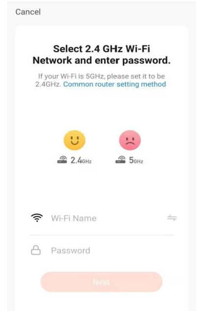
4. Ensure the WIFI light on the air conditioner is flashing twice per second then press on the orange button at the bottom of the screen to confirm
